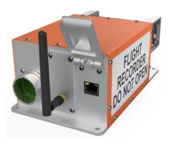
The unit incorporates dual redundant 28VDC power inputs as well as internal Recorder Independent Power Supply (RIPS) as standard to support 10 minute backup.
